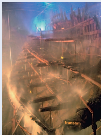
The hull of the Mary Rose , now at the Portsmouth Historic Dockyard (UK), being sprayed with polyethylene glycol solution. Photograph by Farideh Jalilehvand, University of Calgary, Canada.
